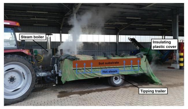
Figure 1 Photograph of the tipping trailer with steaming system, steam boiler and the insulating plastic cover (Photo: P. Dietrich).
